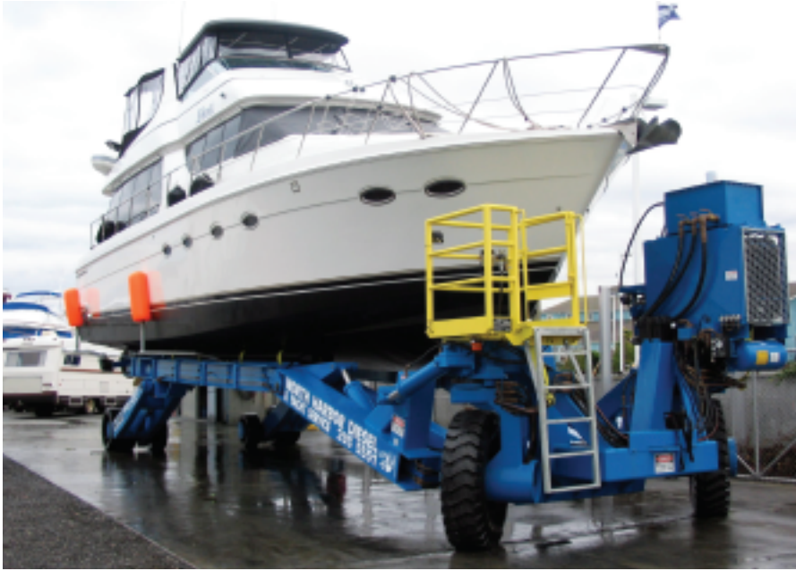
North Harbor Diesel and Yacht Service in Anacortes, Wash., uses a self-propelled hydraulic trailer to move boats from the water to its repair yard, which is 1,875 feet away.
